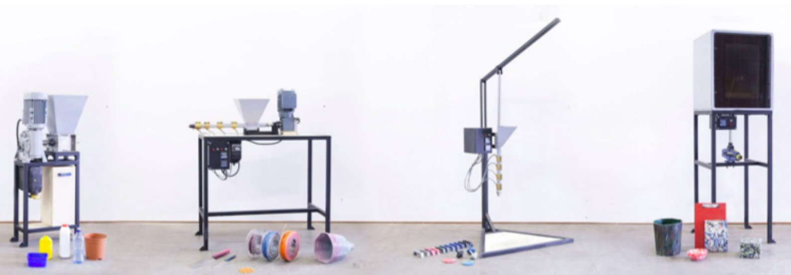
The four machines used in the “precious plastic initiative”
